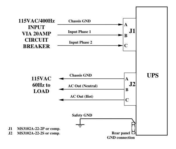
Figure 2 – Electrical Connections
