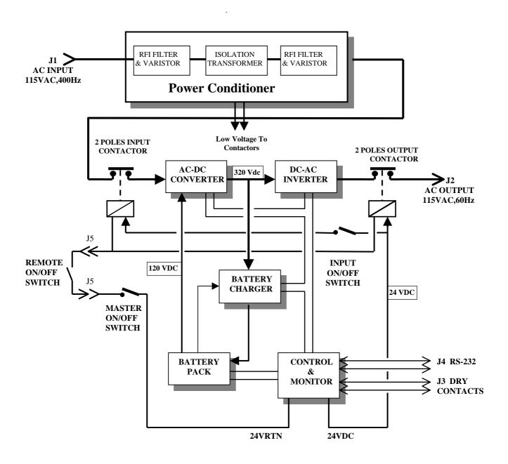
Figure 1: M110BA-2 Block Diagram
