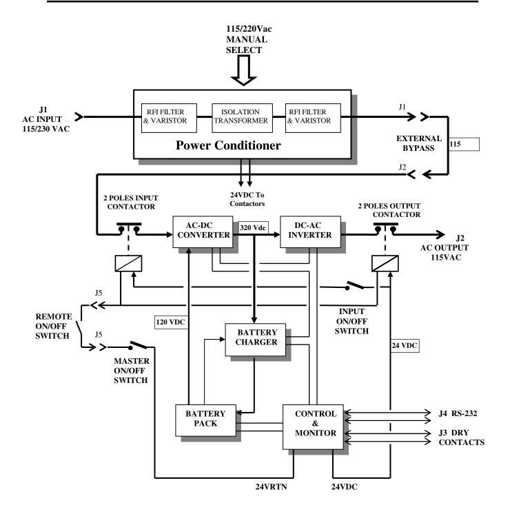
Figure 1: M140BA-1 Block Diagram
